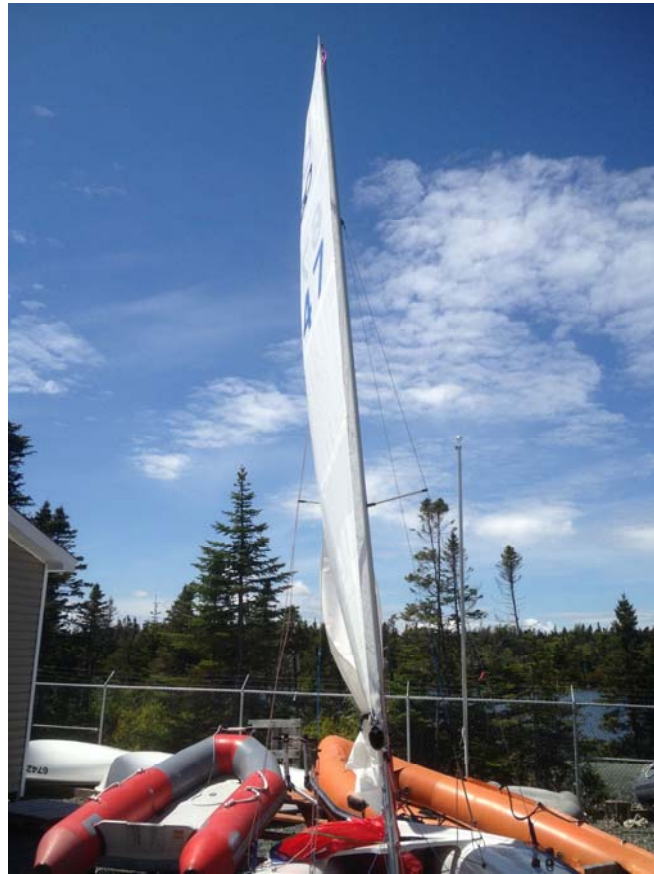
Figure 19 Bladed Mainsail with Bridle Low and Boom Vang and Outhaul Tight
