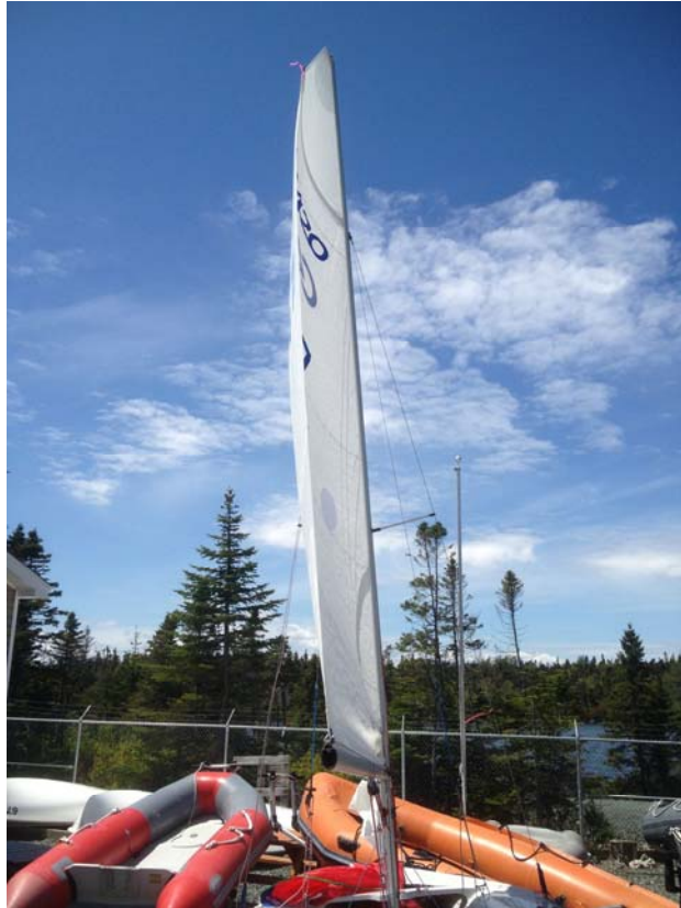
Figure 20 Mainsail Shape for Survival Conditions with Medium Bridle Height with Cunningham, Boom Vang and Outhaul Tight
