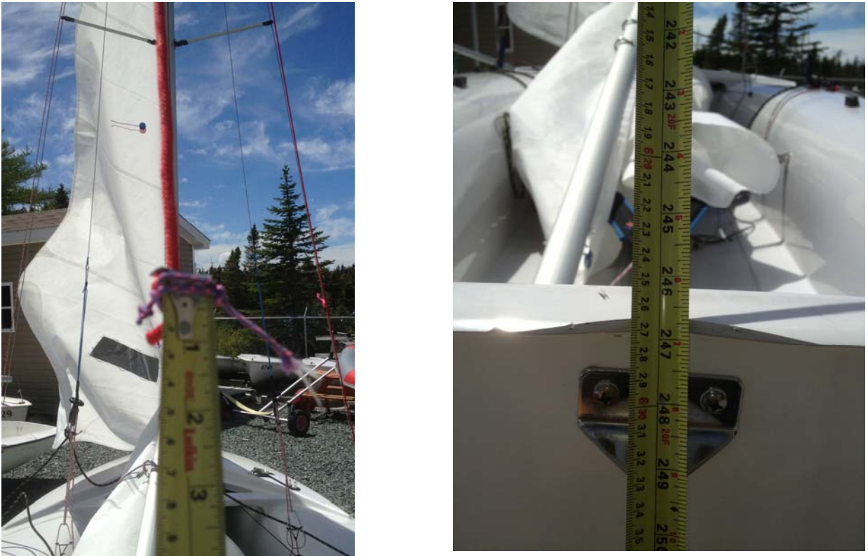
Figure 11 Measure the Rake
