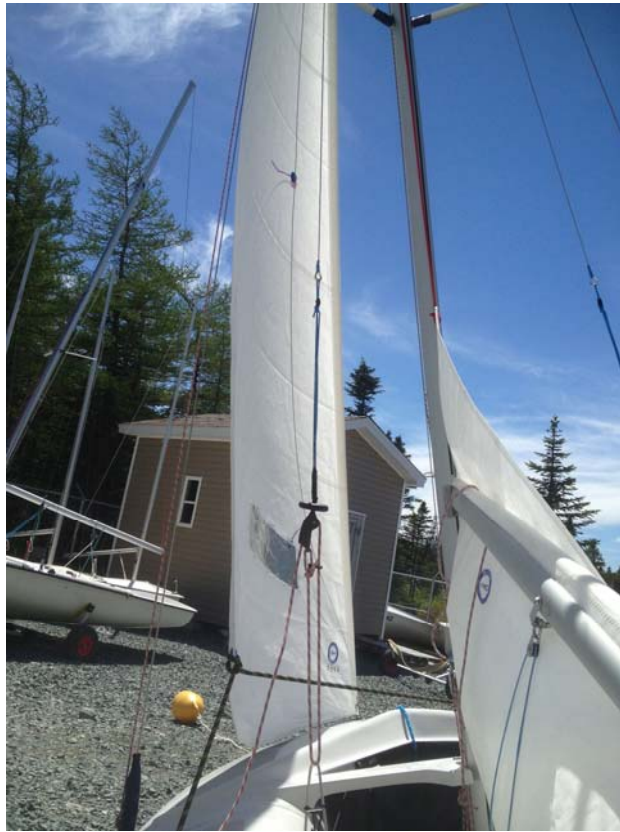
Figure 26 C420 Jib With Correct Windward Sheeting
