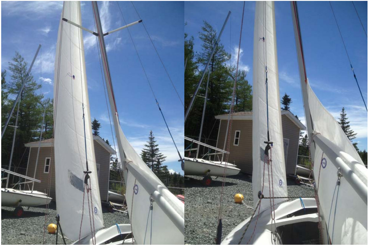
Figures 24 and 25 C420 Jib Without Windward Sheeting & C420 Jib With Excessive Windward Sheeting
