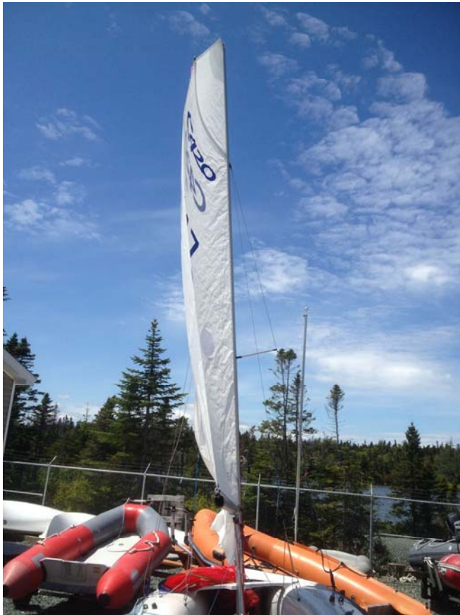
Figure 16 High Bridle Height with Open Leech
