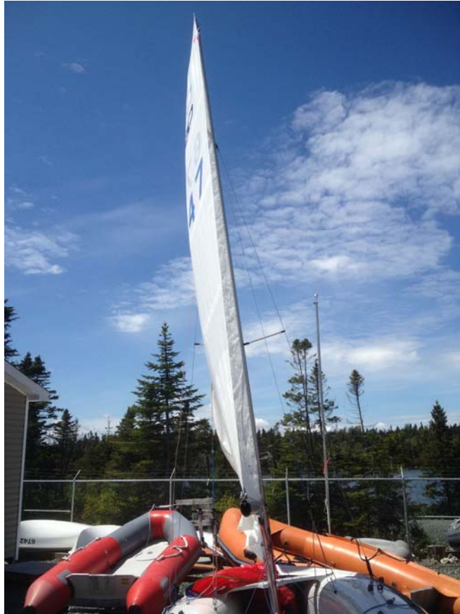
Figure 18 Low Bridle Height with Closed Leech
