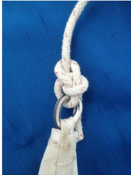
Figure 7 Connecting the Jib Halyard
