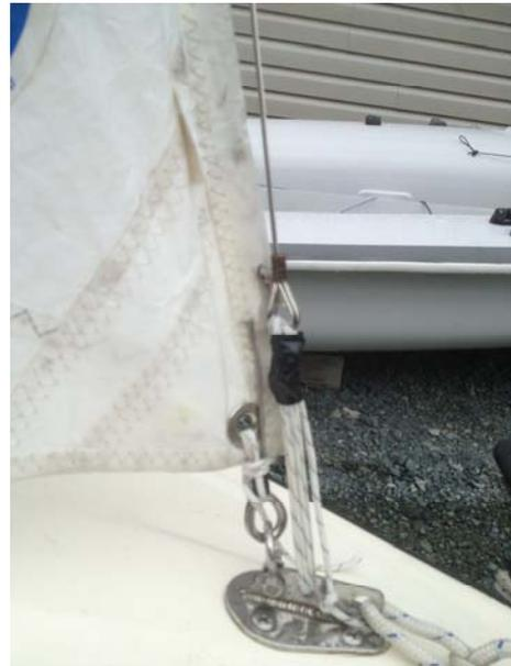
Figure 6 Connecting the Jib Sail
